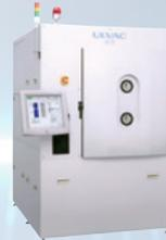
Batch Type High Vacuum Deposition Equipment
